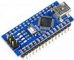
Arduino Nano or Uno (I prefer Nano's because they are small and fit inside props easily)
