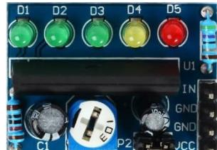
Arduino for signal processing. The 3 wires from this hack need to get to the correct pins or this won't work. On the front the LED's are labeled D2, D3, and D4. They need to end up hooked up as follows: D2 connected to A1 on the Arduino, D3 connected to A2 on the Arduino, D4 connected to A3 on the Arduino.
