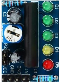
A KA2284 Module this is a small signal meter for audio devices and is the module we are going to hack to get our signal for the jaw to respond to.
